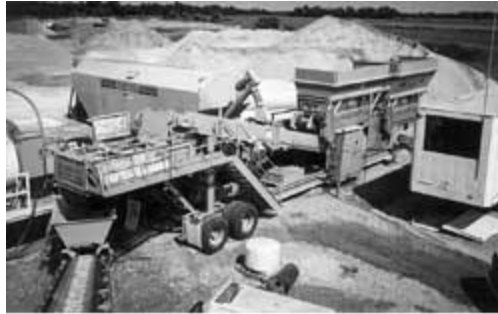
The Kolberg Model 52S features a continuous flow mix and the ability to vary retention time to meet changing job requirements.
