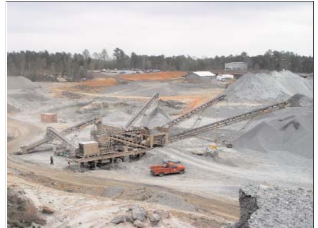
In order to produce more spec stone, Junction City Mining added a portable plant to its tightly organized system of stationary plants.
