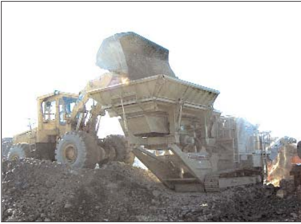
A top size material of 3" x 0" flows from the Pioneer Rocky Trax jaw to a track-mounted screen. The Rocky Trax operates at a 1" closed-side setting. From the jaw, the 1" x 0" material goes to a second portable screen, where three more products are sized, for a total of five products. Production rates for Laurel Aggregates' Rocky Trax are 125 TPH at a 1" CSS in limestone.
