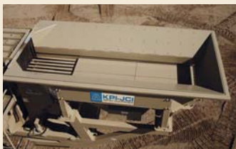
VIBRATING GRIZZLY FEEDER 40" x 14" Vibrating Pan Feeder, 5-1/2 cubic yard hopper with four feet long independant vibrating fingers.
