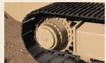
HEAVY DUTY TRACK DRIVE 400mm tracks with dual drive. Heavy duty track drive provides extreme durability and mobility.
