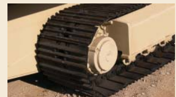
TRACK MOUNTED CARRIER Designed for 3/4 MPH speed at full throttle. Transport on standard low-boy.
