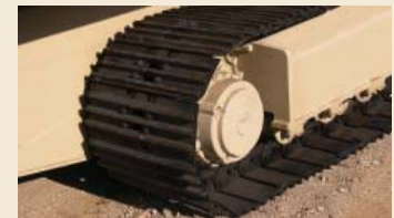
TRACK-MOUNTED CARRIER Tracks provide both jobsite mobility as well as the foundation required to isolate plant vibration.
